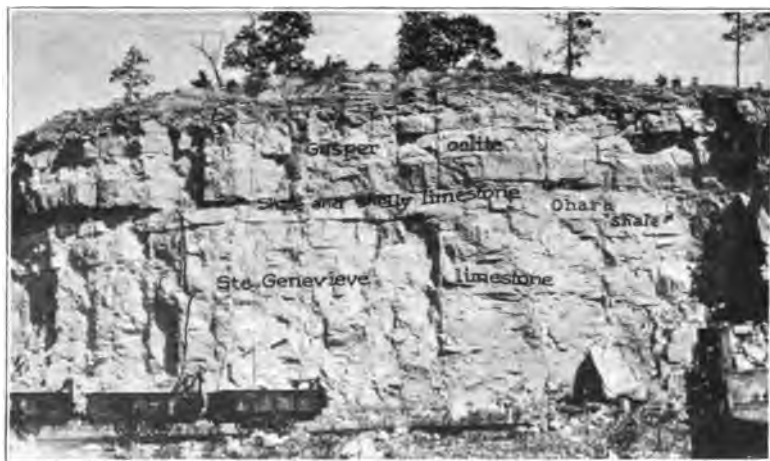
Plate 75. Quarry one-half mile west of Carter, Carter County. Looking north Ste. Genevieve limestone and Gasper oolite. The succession from the base up is limestone full of small quartz pebbles, shale, limestone, shale, thick-bedded Gasper oolite, and thin-bedded dark limestone at top of quarry face. Green shale overlain by massive limestone above top of face. The yellow layers of the Gasper and the gray layer between are very distinct. Lower yellow layer with Martinia contracta . The limestone here is probably a thickened representative of the Maxville limestone of Ohio.
